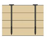
screw: TBSF8149 timber element: 4 x 38 mm (1 1/2") total thickness: 152 mm (6 ")
